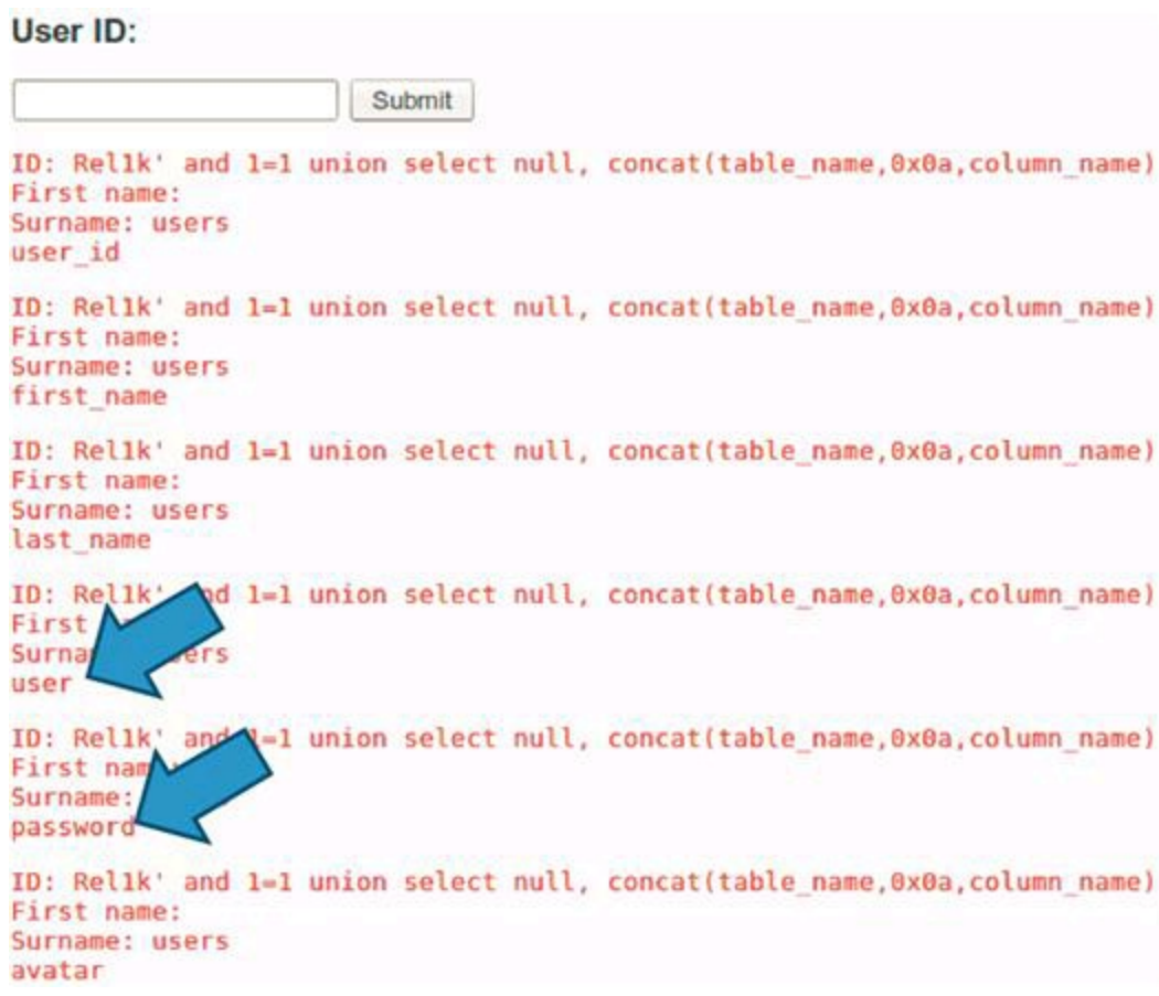
FIGURE 4.6 Results from injection accessing the information schema for the “users” table.
