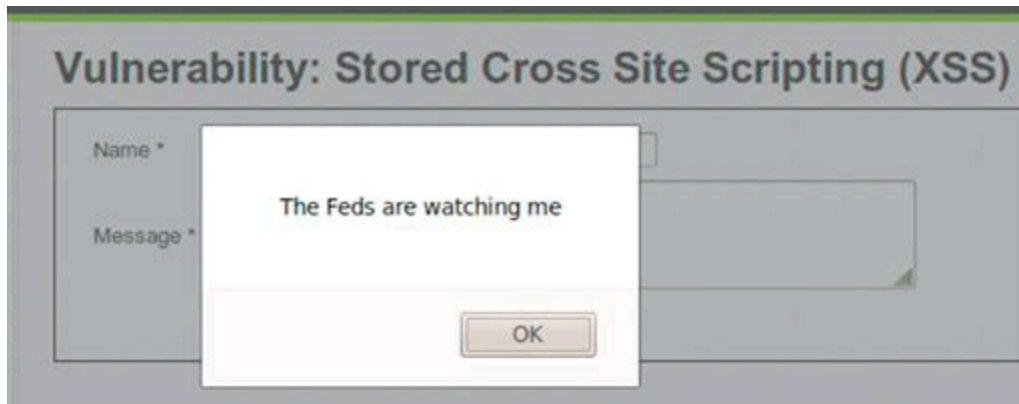
FIGURE 6.13 Output of stored XSS attack in DVWA.
