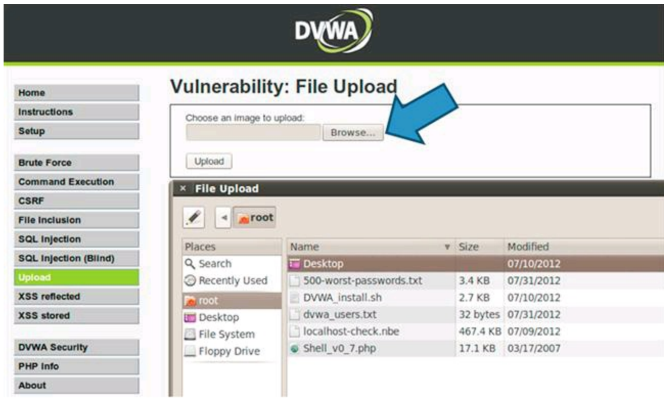
FIGURE 4.17 Uploading a web shell to the DVWA web server.
