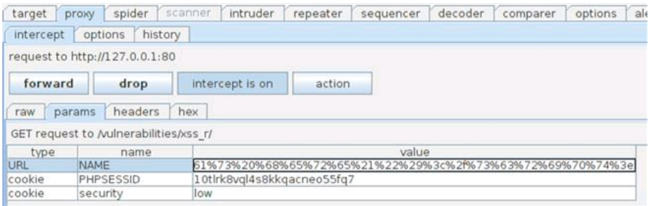
FIGURE 6.8 Using URL-encoded XSS attack in Burp Proxy.
