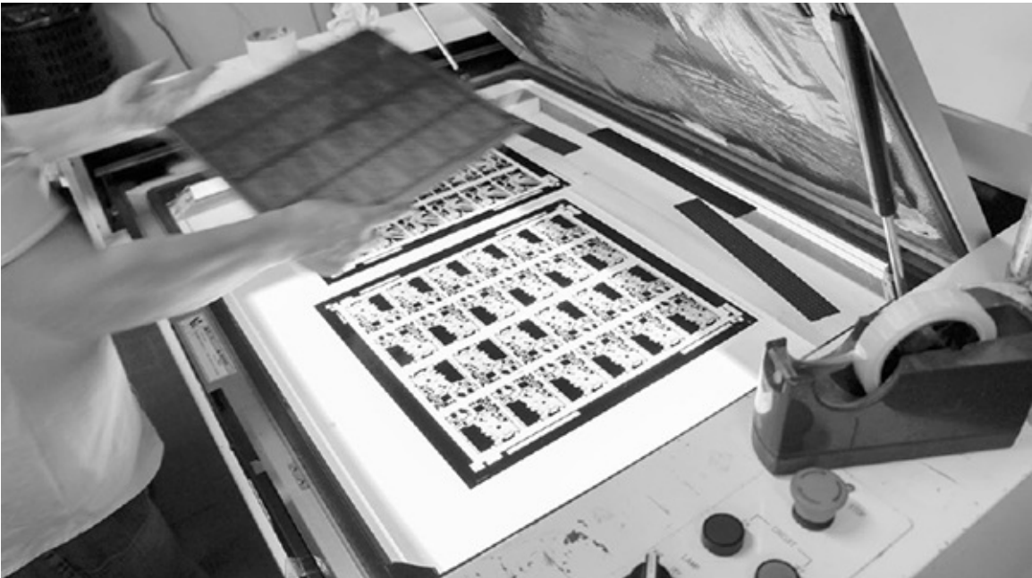
A PCB being mounted into a light box that will expose its unprocessed backside film
