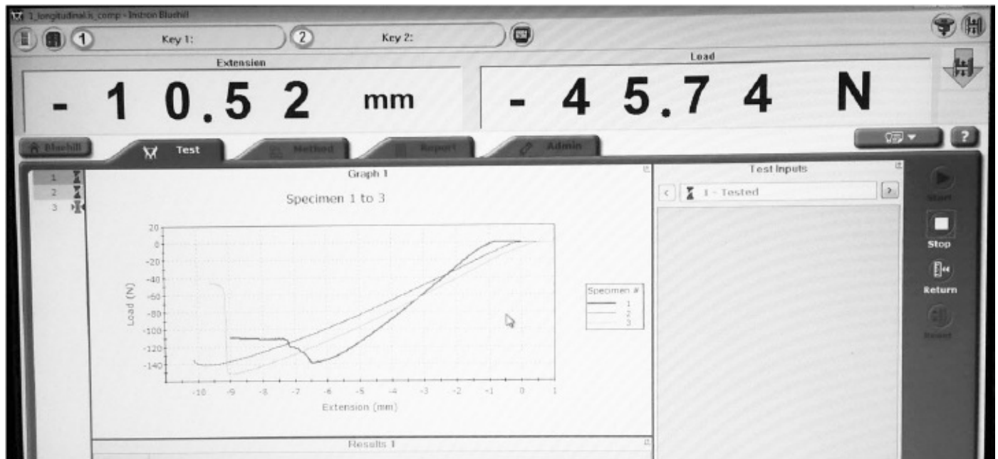
Graphs of load versus extension on the Heirloom laptop composite, as plotted by the Instron testing machine
