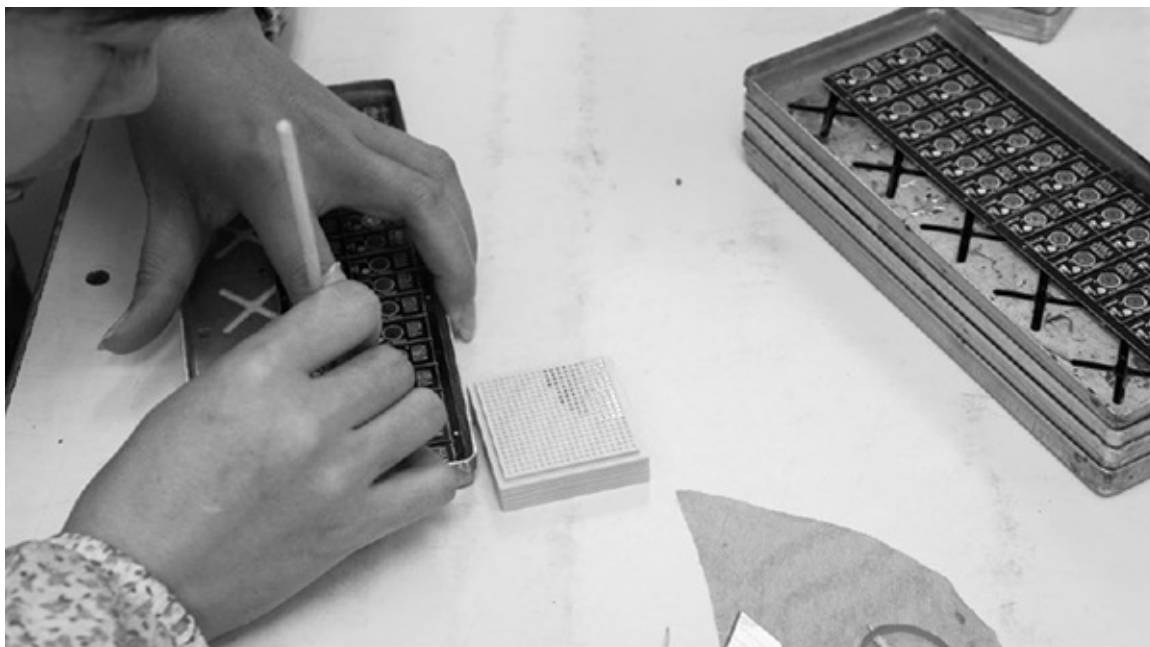
A controller IC being placed on a panel of USB-stick PCBs. The tiny bare dies are on the right, sitting in a waffle pack.
