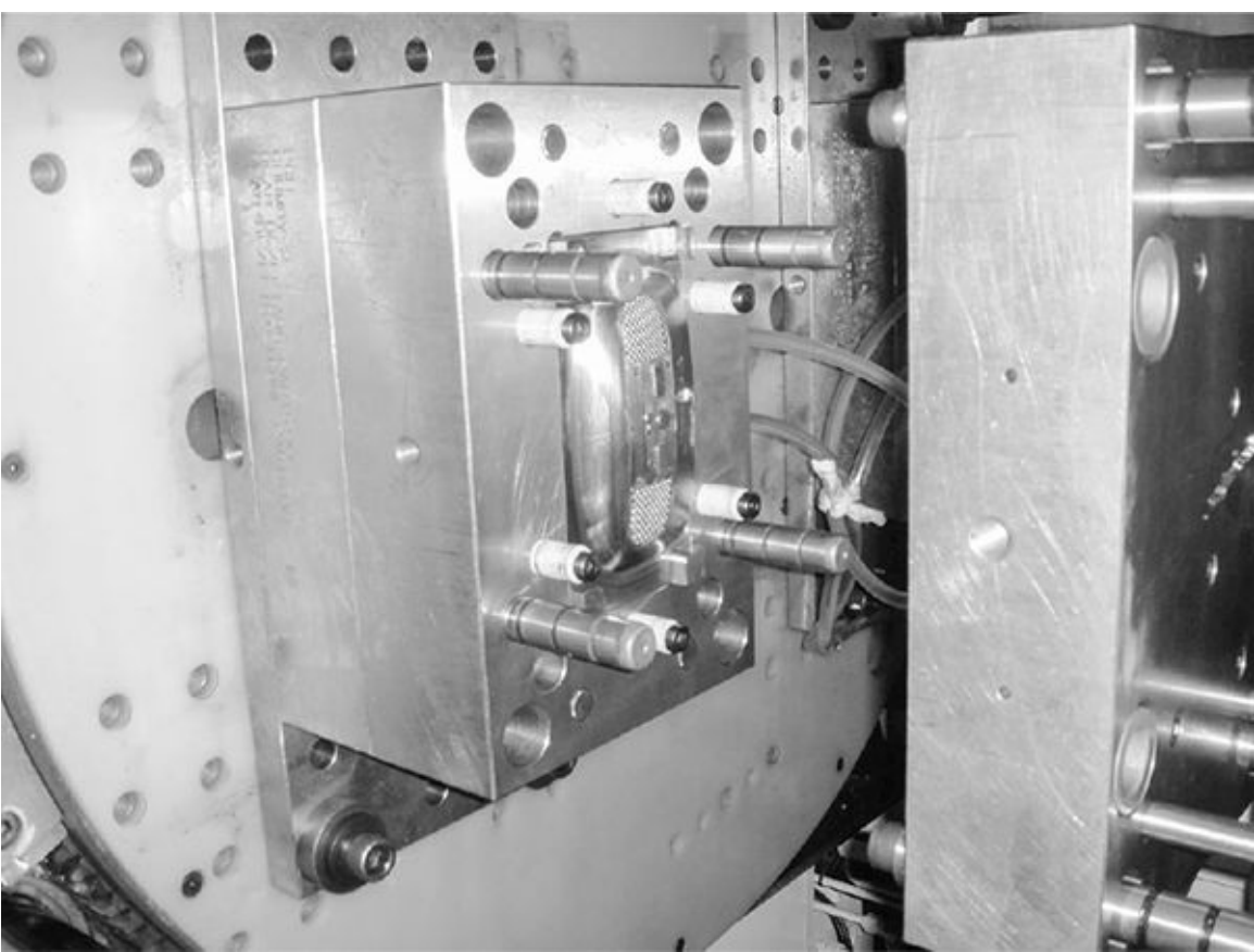
The final mold for the chumby's back bezel, inside an injection-molding machine
