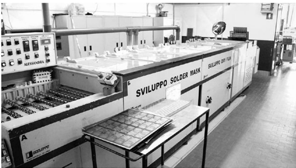
The machine that develops the photoresist
