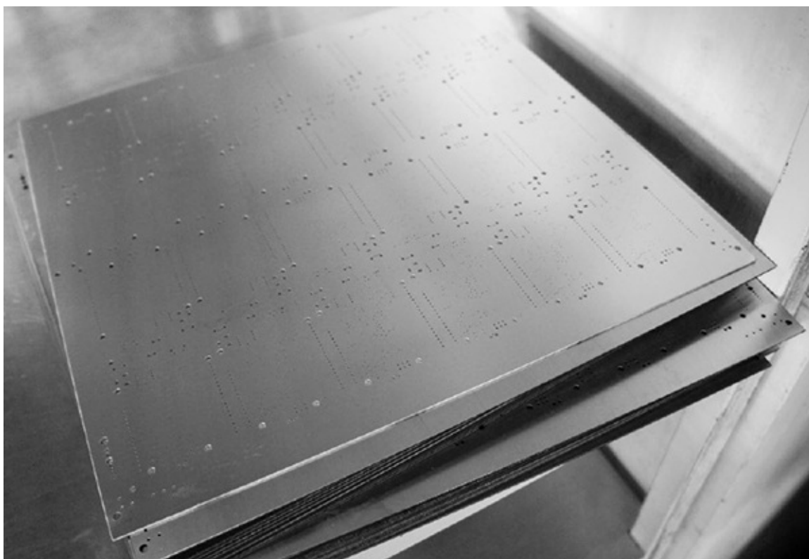
A stack of finished, drilled panels of Arduino Leonardo boards
