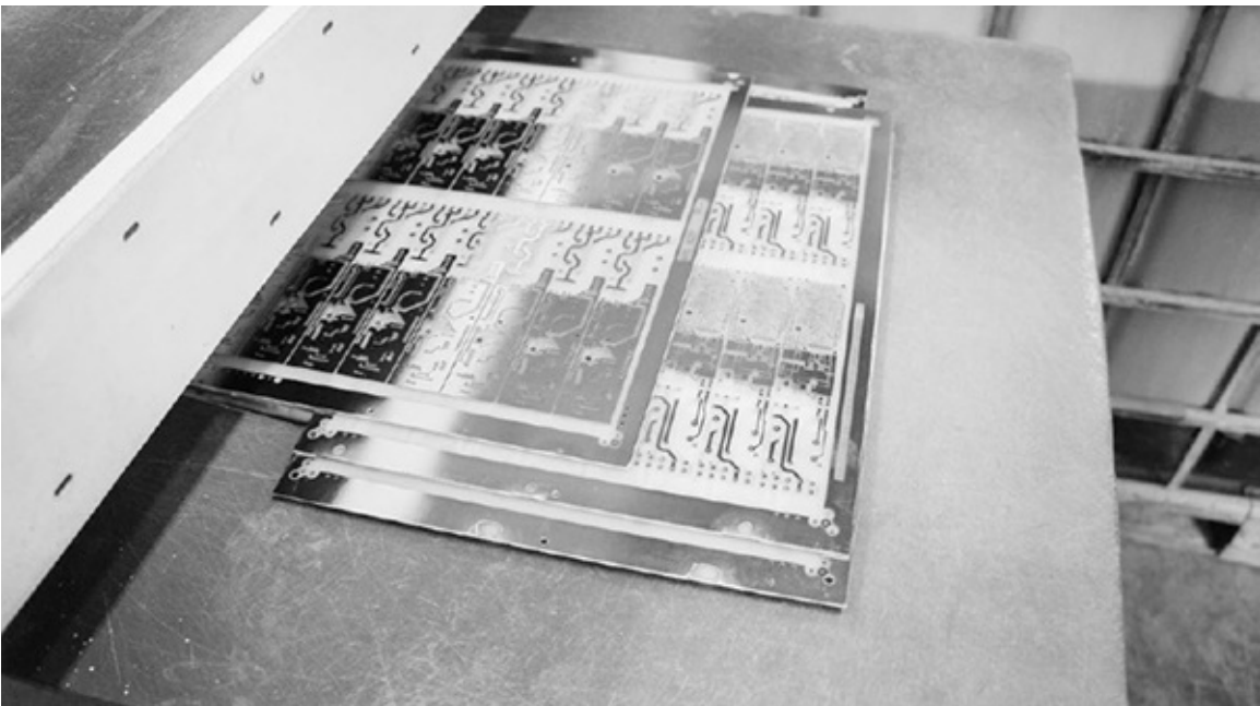
PCB panels with bright, shiny copper. This photo doesn't show an Arduino panel, as those weren't going through the machine when I photographed it.
