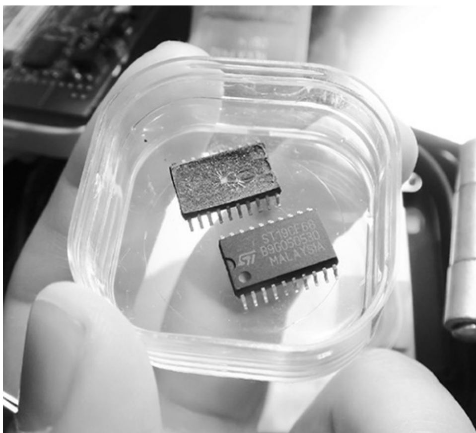
Two suspicious chip specimens from an Asian source
