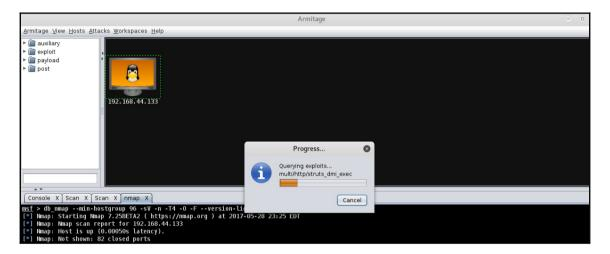
Once the Armitage console finishes querying for possible exploits, you can see the list of applicable exploits by right-clicking on the host and selecting the **Attack** menu. In this case, we'll try to exploit the postgresql vulnerability as shown in the following screenshot:
