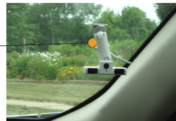
CAMERA Mount to passenger side windshield a few inches above the dash or midway up the pillar.
