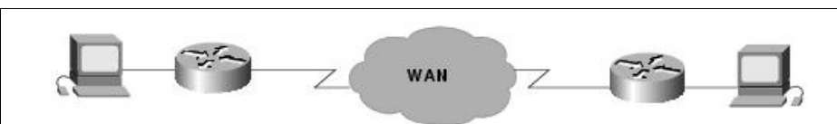
Figure: A Typical Point-to-Point Link Operates Through a WAN to a Remote Network
