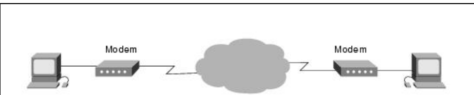
Figure: A Modem Connection Through a WAN Handles Analog and Digital Signals
