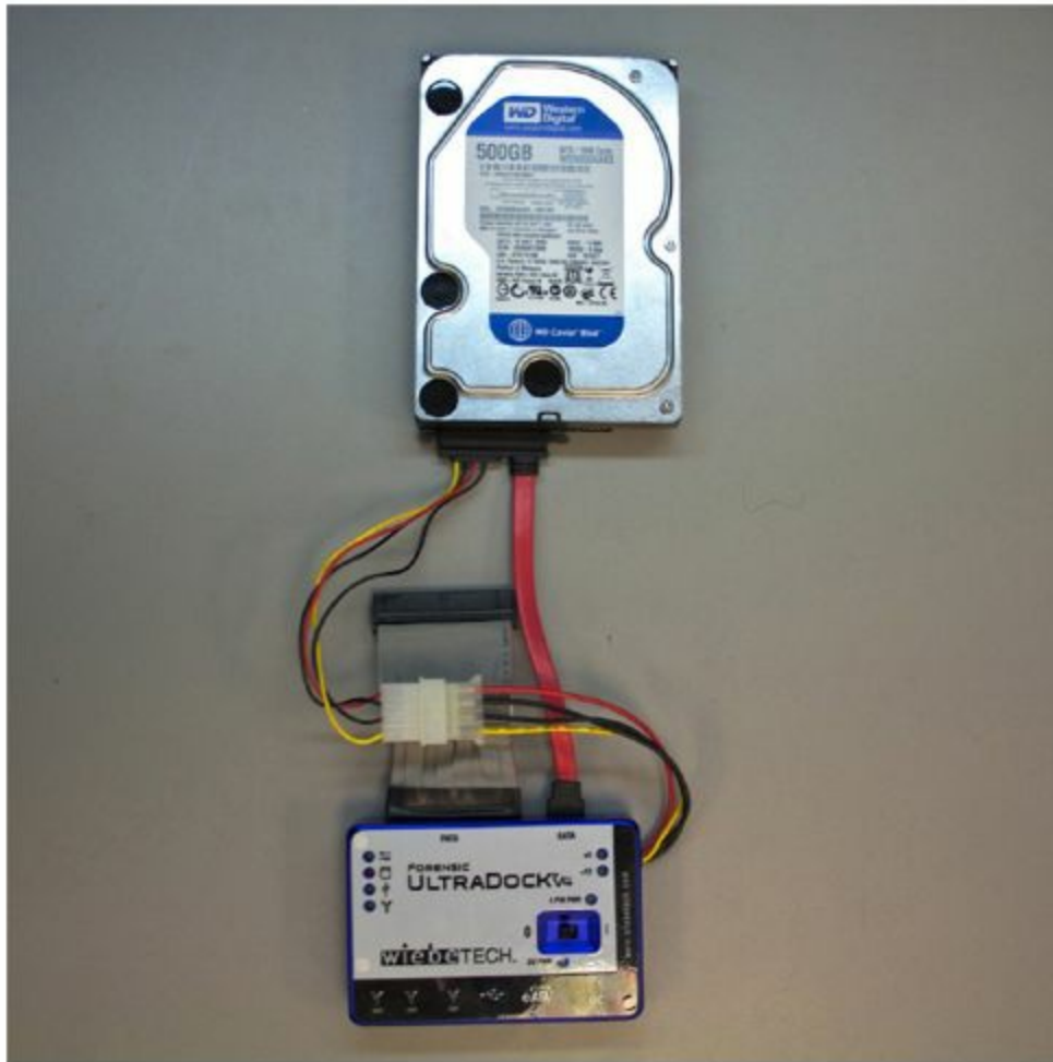
Figure 8-3. eSATA write blocker hardware
