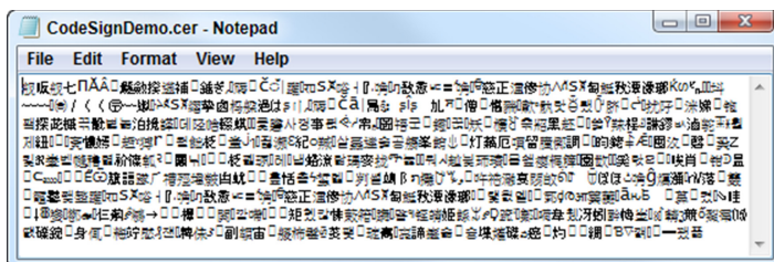
Figure 9-3: Binary encoded DER (.cer) certificate format
