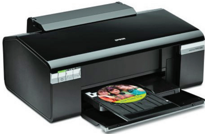
Figure 4-6: Inkjet printer for printing on flat surfaces
