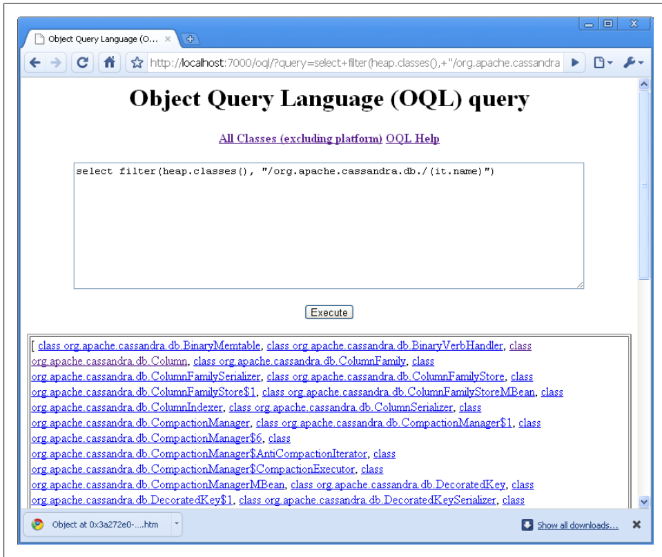
Figure 9-8. Using Object Query Language in JHAT to filter only Cassandra's classes in the db package
