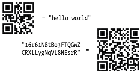
Figure 2-1: QR codes can be used to represent arbitrary data. They are easy to scan with smartphones and so are convenient for sharing the long strings of characters used for Bitcoin addresses.
