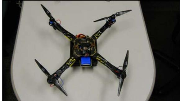
The quadcopter has two sets of counter-rotating propellers, which simply means that two of the propellers rotate clockwise and the other two rotate counter-clockwise to provide thrust in the same direction. This provides a platform that is inherently stable. Controlling the thrust of all four motors allows you to change the pitch, roll, and yaw of the device. The following is an image that may be helpful:
