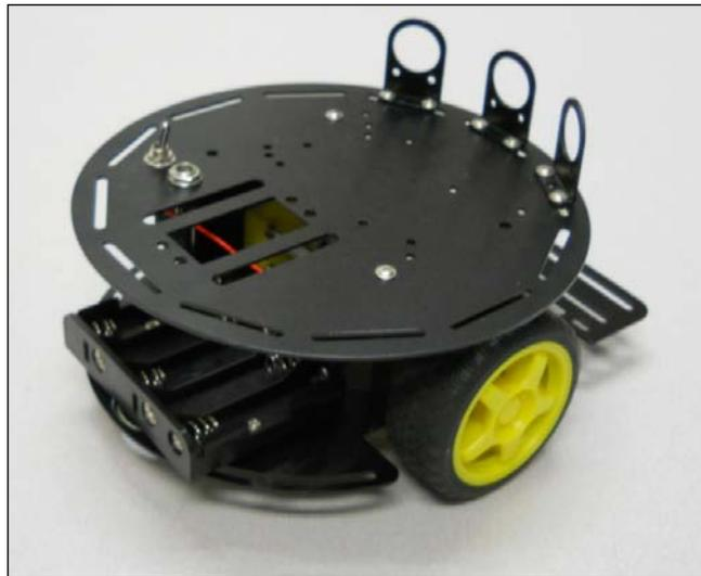
To make this wheeled robotic platform work, you need to control the two DC motors connected directly to the two wheels. You'll want to control both the direction and the speed of the two wheels to control the direction of the robot.
