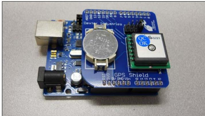
You can use the pin labels to match the pins on Arduino. Now, it is securely on top of your Arduino device; let's look at how to access the device via the SW.
