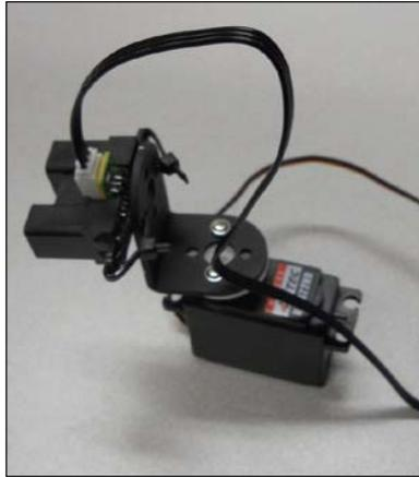
You'll need to connect both the IR sensor (as described earlier in this chapter) as well as the servo to Arduino (as explained in *Chapter 7, Controlling Servos with Arduino*).
