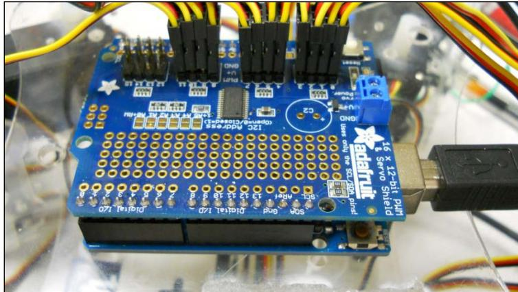
This particular shield can handle up to 16 servos. The important characteristic of this servo shield is the connection on the right-hand side of the shield. In the GND and VCC connections, you'll place your external voltage and current input, allowing Arduino to control many more servos.
