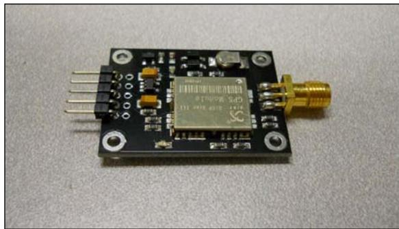
Fortunately, this unit comes with its very own antenna, and you'll connect this to the RF (gold) connector on the board. This particular device interfaces using the I2C interface, one that your Arduino supports. In order to connect the device, you connect the pins to the board. The following is an image of these pins:
