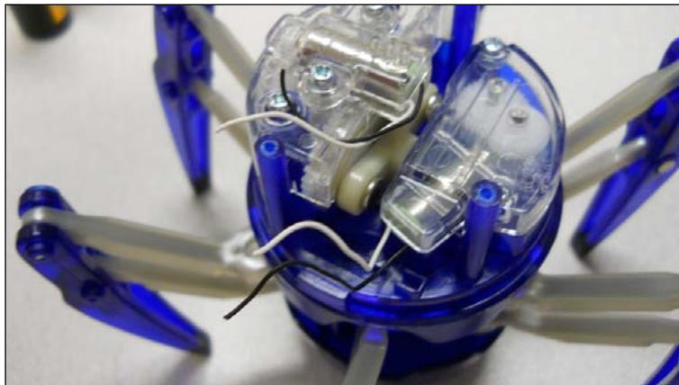
2. You'll want to add extension wires onto each of the six wires, so you can connect them to the TinyDuino that you'll mount on top of the robot. Once you have done this, route these wires out the hole to the left by removing the small controller board, and then reattach the top of the robot and the top plate.
